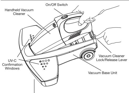
Bulb Protection Cover & UV-C Bulb Under Unit
